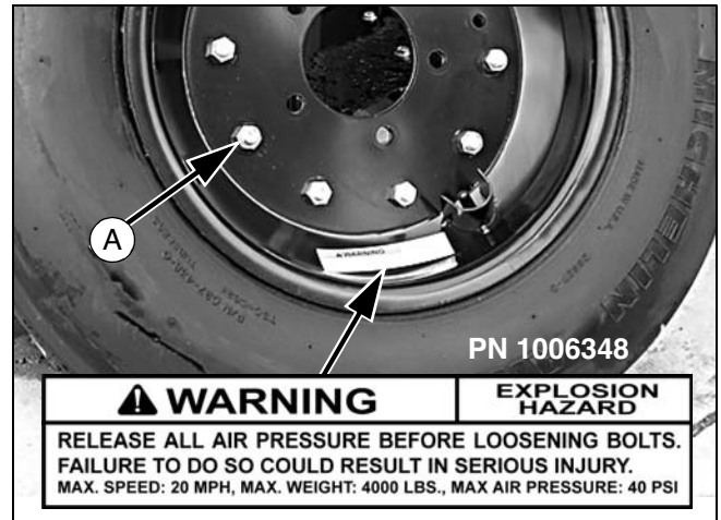
Figure 9. Split Rim Tire Servicing
