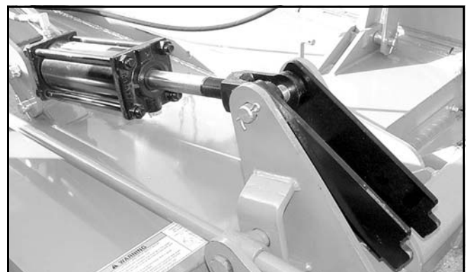
Figure 4. Transport Lock In Operation Position
