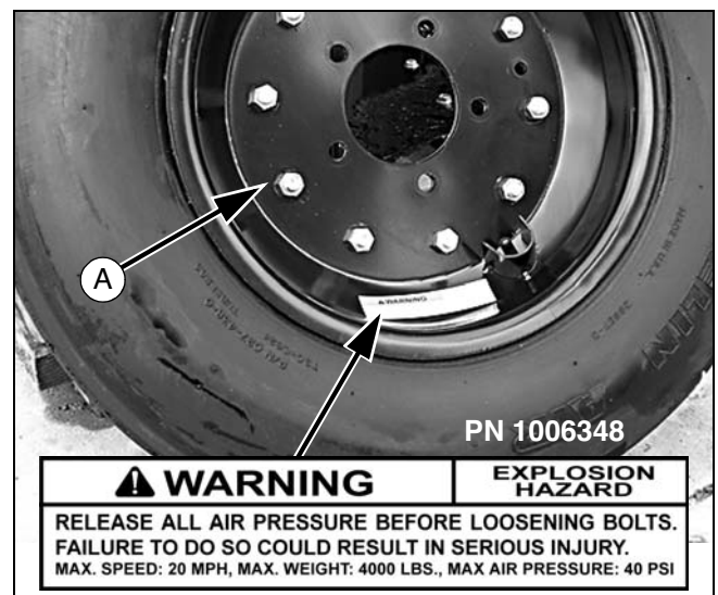
Figure 21. Split Rim Tire Servicing
