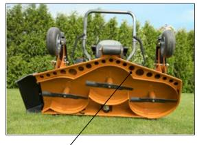
MXV-Baffle™ creates strong suction, lifting grass for a precision cut and keeping dust under the deck.
