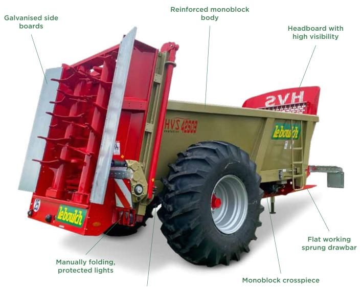
Transmission under the axle for the lowest point of gravity on the market
