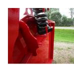
Tension springs have six adjustments to set angle of screen and tension on the screen assembly.
