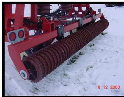
5 bearing main frame section, lights & reflectors standard
