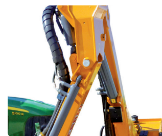
Hydraulic breakaway on second arm with accumulator controlled autoreset facility.
