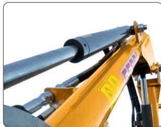
Arm with circular section H.T.R. (High Torsion Resistance).
