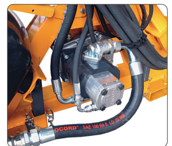
Group 3 cast iron hydraulic rotor pump.
