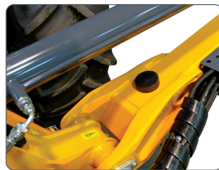
Drop forged arm brackets.
