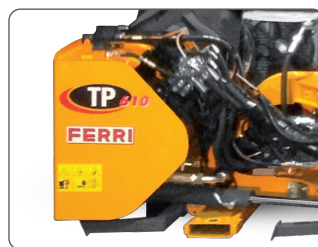
New design bolt on and pressurized oil tank (Classic).
