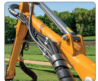
Arms with circular section H.T.R. (High Torsion Resistance).
