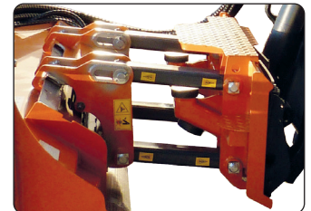
Parallel linkage for better floating on uneven grounds
