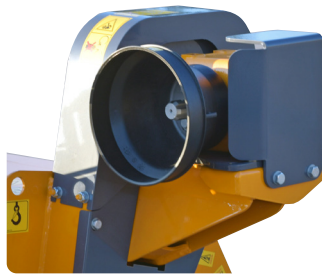
Gearbox unit outside the transmission cover (more offset and less PTO angle).
