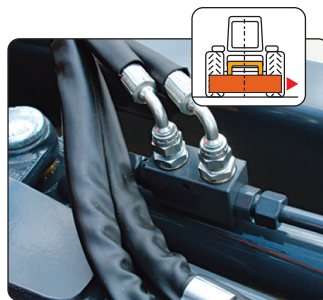
Hydraulic block valve for transport with automatic activation (no chains or holders).
