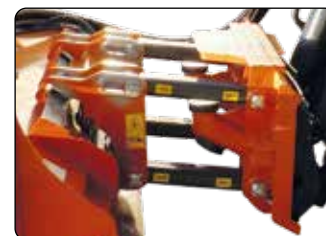
Parallel linkage for better floating on uneven grounds
