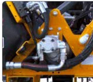
Aluminium rotor drive hydraulic pump.
