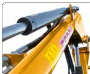
Circular section of the arms H.T.R. (High Torsion Resistance).
