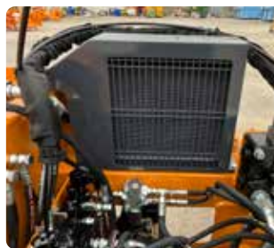
Oil cooler with thermostat.
