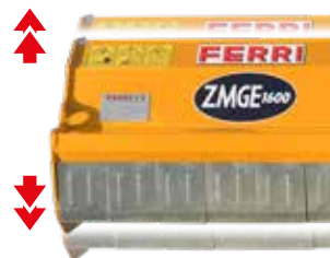
Floating frame following the ground contours
