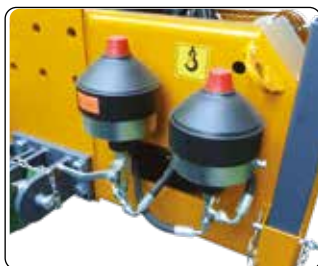
Lift float nitrogen accumulator.
