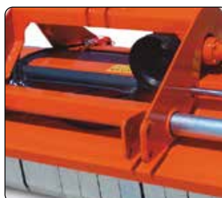
Side shift linkage with hydraulic cylinder.
