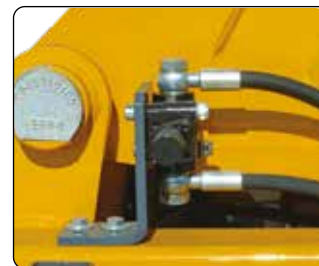
Single acting- double acting automatic switch.
