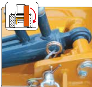
Mechanical block pin for transport (no chains or holders)
