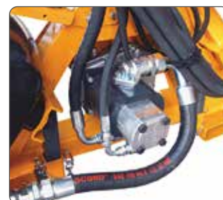
Group 3 cast iron hydraulic rotor pump.
