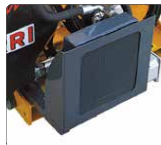
Oil cooler with thermostat (option).
