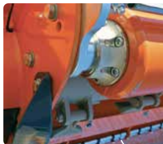
Rear roller support with internally fixed bearings NG without grease fittings.
