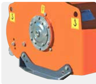
Rotor support with bearings positioned inside the frame.
