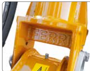
Drop forged parts for arm linkages.
