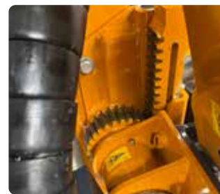
Rear mounted flailhead with rack and pinion gear to ensure the most precise cutting position.
