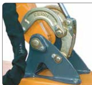
Drop forged lever for flail head rotation.
