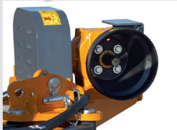
Gearbox external to the drive housing.
