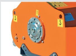
Rotor support with bearings positioned inside the frame
