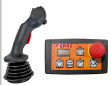
Proportional electrical control with electric rotor management. The EG Tronic control allows for easy portability of the cab control thanks to a light joystick and the lack of hydraulic hoses. The joystick is connected with an electrical cable to a control unit mounted on the distributor valves. The action is precise for cross movements of the first and second booms. The rotation direction of the rotor is controlled by electric switches on the console.
