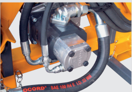
Group 3 cast iron hydraulic rotor pump
