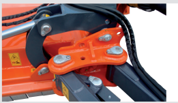
Rotation joint on self lubricating bushing.
