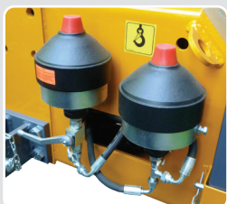
Lift float nitrogen accumulator.
