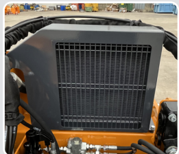
Oil cooler with thermostat.
