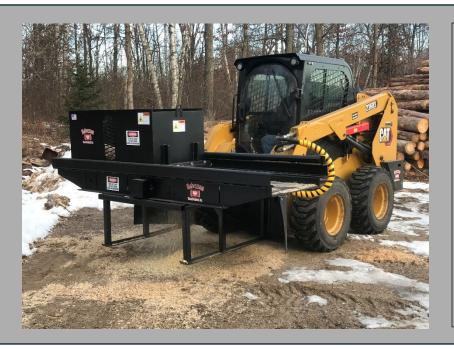
Perfect for residential and farm use, the HWP- Shuttle Shaver truly makes the job hassle-free. When attached to a skid steer or other machine, it enables one person to easily and efficiently produce high quality bedding. Make your bedding as you need it! This shaver turns your logs into quality shavings for your animals and poultry. The mobility and efficiency of this shaver is a time saver!
