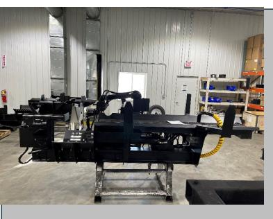
Perfect for commercial use, the HWP-160 truly makes the job hassle-free. When attached to a skid steer or other machine, it enables one person operating it to easily and efficiently perform wood cutting and splitting tasks. All from the comfort of the cab. Take the processor to the wood, instead of having to bring the wood to the processor! The mobility and efficiency of these Firewood Processors is a time saver!
