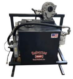
PTO Pump Speed: Hydraulic Specifications: Hydraulic connections: Hydraulic Cooler: Cooler Fan: Assembled Weight: Assembled Dimensions: Shipping Dimensions: Connection Method: Oil Tank Capacity: Leg Style: Warranty: 540 RPM 21.2 gpm @ 2500 psi (maximum) 2 (Includes a port for adding case drain) 50 GPM 12 Volts 168 lbs. (Dry) 31.25" x 30.25" x 20" 35" x 34" x 25" 3-point hitch 25 US Gallons Adjustable 6 Months
