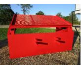
Screen with  $\frac{3}{4}$ " openings has two centre flat bar hold-downs and two angle iron hold-downs on each side to prevent run-off.
