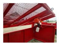
Oli vibrator 110V standard, purchaser to complete electrical wiring for their requirements and local codes. Can be operated with 110 extension cord, generator or inverter.
