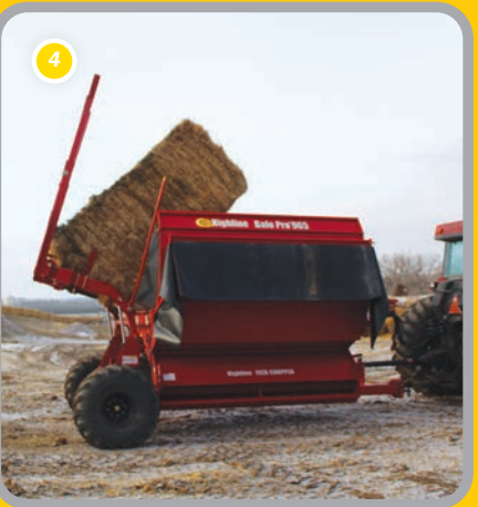
The Twine Sickle™ cuts the twine and the bale is dropped loosely into the tub (the loose consistency helps with uniform processing).
