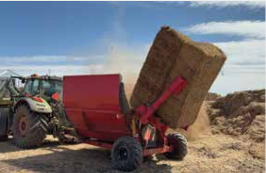
Loads large square bales lengthwise.
