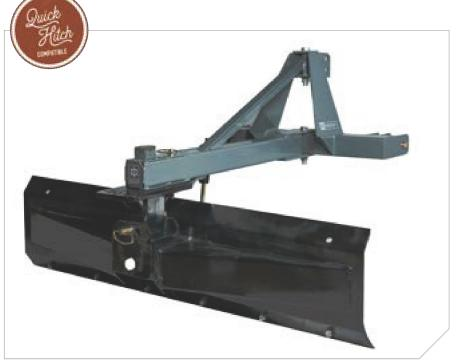
These Heavy-Duty Grader Blades are IronCraft's toughest grader blades. These models will easily meet all of your land grading, leveling, or backfilling needs. Designed for 50 to 75 hp tractors, they feature a five-position angle adjustment, three-position tilt adjustment, utilize a ratchet jack for the offset adjustment, and are Category I & II quick hitch compatible. Three models provide working widths from 72" to 96".
