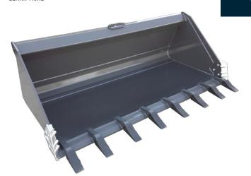
Designed for the most demanding track loaders on the market. 1" x 8" cutting edge, 1/2" AR400 heel plate and 1/2" wear bars, reinforced quick attach, ¼" bucket wrap, rolled back for easy clean out. 65 HP and over. (Image shown with optional teeth and optional side cutters)
