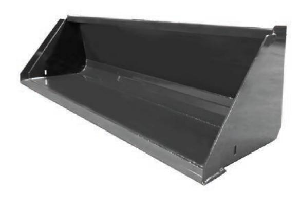
Our tractor buckets are designed with higher backs to prevent material from spilling over. They feature 3/16" steel sides and a 3/4" x 6" cutting edge. These buckets also come with holes in the sides for mounting a tooth bar and will hookup using universal Skid Steer and many tractor styles quick attach.
