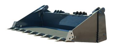
The cylinders on our Heavy Duty 4-N-1 Buckets have a 2.5" bore. They are equipped with a 1/2" x 6" cutting edge and 1/2" x 4" at all other ground engaging points. They are built with top quality steel, oversized pins and bushings, with grease fittings at every pivot point. Every unit exceeds the lifting capacity of the skid steer machine it is used on. Optional weld-on teeth available.
