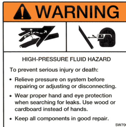
# 8 – WARNING HIGH PRESSURE FLUID HAZARD Part # 224-02
