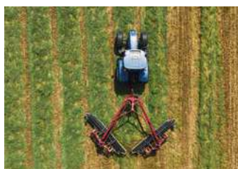
Basket Rake in the work position.
