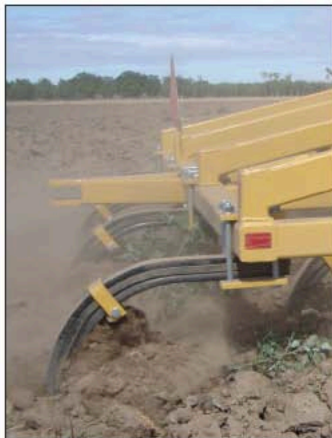
Triple Shank Assembly is standard on all 3-Bar models
