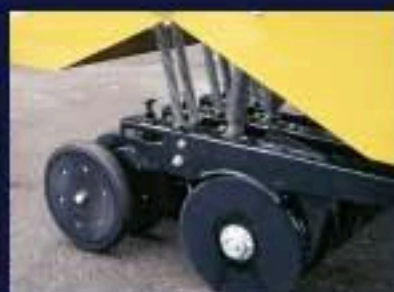
Rugged double disc opener with "T" handle adjustable presswheel
