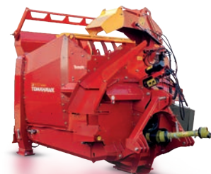
TOMAHAWK 8250 | M CAPACITY 113 ft 3 Distance : 65ft Tractor : 150HP (min.)
