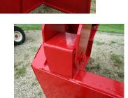
Screen hinge pins mounted in rubber blocks (use of isolating rubber mounts reduces vibration loss through main frame keeping as much vibration on the screen area as possible)
