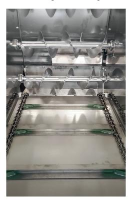
This same "farmer-driven" change has happened with the stainless steel auger flighting. Introduced in 1988, the stainless auger is now firmly in place as the preferred auger; all carts built have at least some stainless augers, and the majority of the carts have all augers made with stainless steel flighting.
