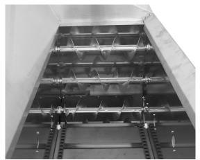
A hinged shield provides easy access to heavy duty drive belts and chains.
