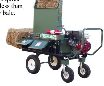
Equipped with the powerful, smooth-running twin cylindar 16 HP Briggs-Vanguard engine, the KB1250 is an excellent choice for fast chopping of newspaper and other demanding material.
