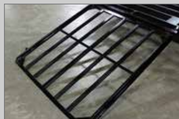
SUPER HEAVY-DUTY REAR RAMP DOOR 5500# CAPACITY, 7500# OPTIONAL
