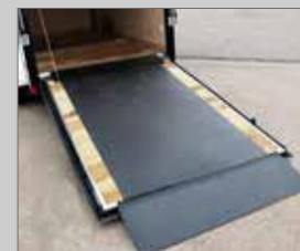
ROCKGUARD COATED STEEL TREAD PLATE ON RAMP AND REINFORCED STEEL FLAP
