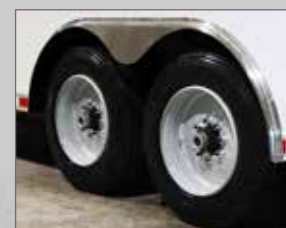
HEAVY-DUTY OPTIONS, 12K NOSE JACK AND UP TO 8K AXLES
