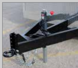
HD 54" A-FRAME WITH ROCK-GUARD COATING
