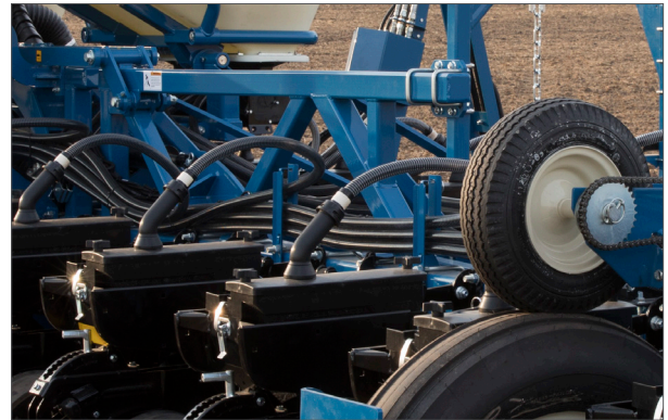
3605: Frame is reinforced with truss style framework with external vacuum manifold.
