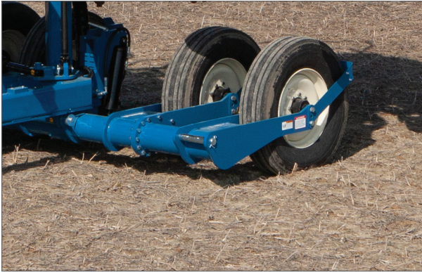
3665: Rock shaft style axle is used to raise planter at end of field.
