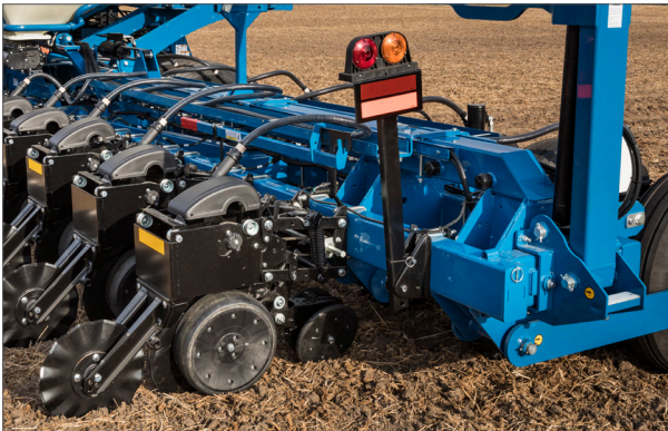
3665: Frame is reinforced with top tube that also functions as the vacuum manifold.
