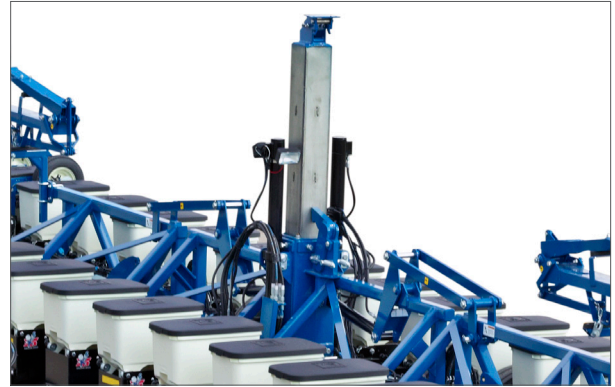
3605: Center post is used to raise planter at end of field.
