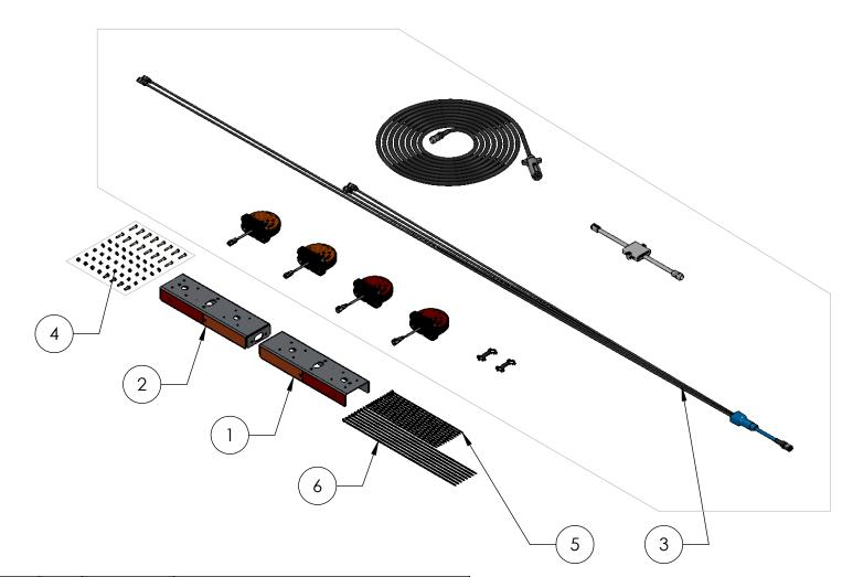
ITEM QTY. PART **DESCRIPTION** NUMBER NO Bracket - Light Mount Assembly A002396 (Right) (Black) Bracket - Light Mount Assembly A002397 (Left) (Black) Lighting Kit - Safety Flashing (w/Lights) (01-6657-T9) K000165 3 K002166 Kit - Light Mount Hardware 4 12 P000152 Cable Tie - 15" x 50# Black 5 8 P002468 Cable Tie - 24" x 80# Black 6
