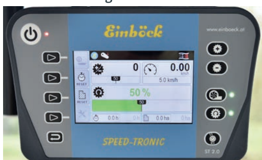
The operation terminal of the STI controller
