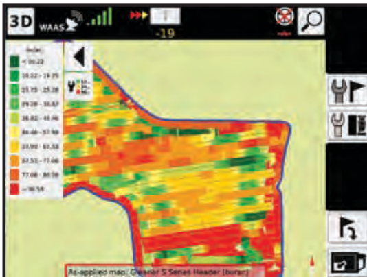
Gleaner Tyton terminal screen showing FieldStar Live real-time yield mapping.
