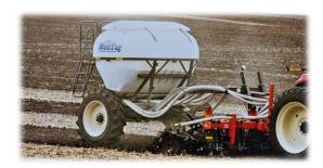
6-Ton GEN I Base Unit with a white bin on a Montag Auto-Steer Cart shown above. Other color options include gray and yellow (see image below). Bins have two fill inlets. All units use the Montag GEN I particulate metering technology.
