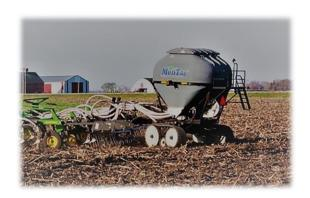
9-Ton GEN I Base Unit with a gray bin on a Montag Auto-Steer Cart shown above. Other color options include white and yellow (see image below). Bins have two fill inlets. All units use the Montag GEN I particulate metering technology.
