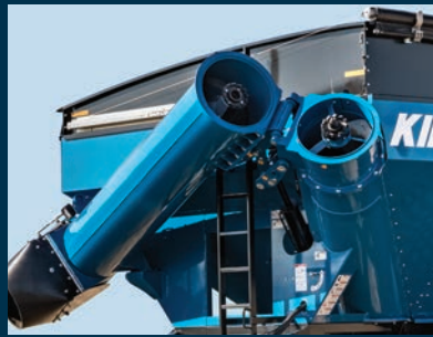
Front folding corner auger for excellent operator visibility
