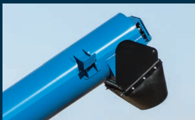
Precise grain placement with standard 35° adjustable spout
