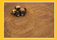
Shift into smooth. The CAT® 16-speed Powershift transmission keeps you moving with 8 gears in the working range and a transport speed of up to 24.6 MPH. You'll immediately notice its smoother shifting and better control with the inching pedal. The result: less operator fatigue.
