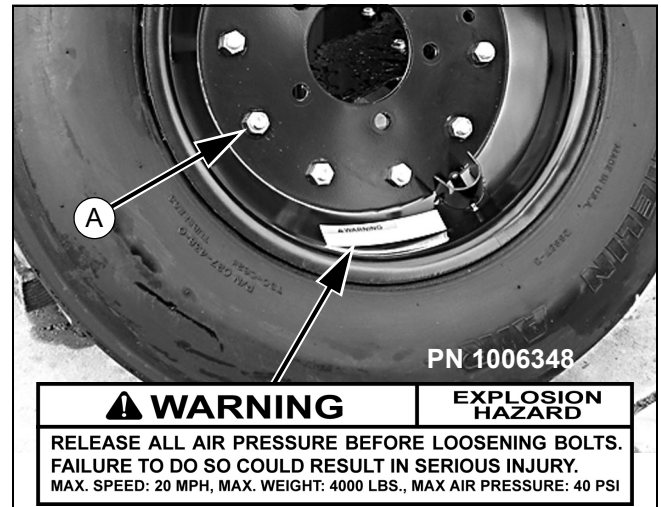
Figure 10. Split Rim Tire Servicing
