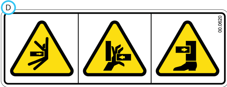
Pinching or crushing hazard.
