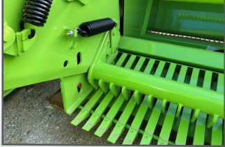
Heavy duty batt springs, 450 BNH steel reel and grate with replaceable teeth
