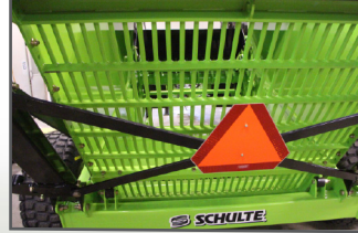
Rear and bottom grates ensure soil is easily sifted through the hopper
