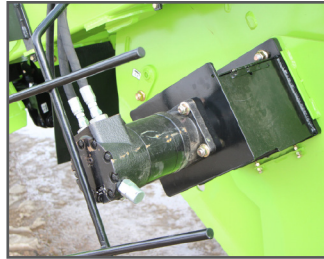
All hydraulic motors have a built in cushion valves for longer life
