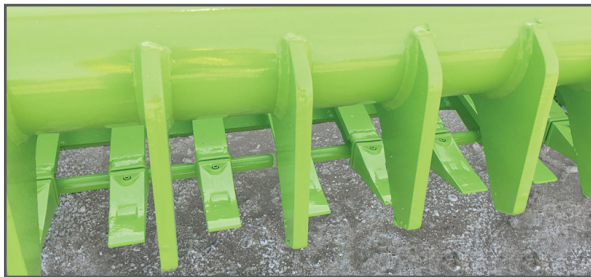
450 BHN steel for heavy duty windrowed picking
