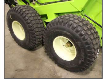
Tandem walking axles with 16.5L X 16.1 X 10 ply flotation tires
