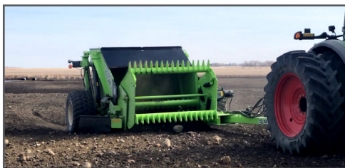
Wide grate for minimum till picking
