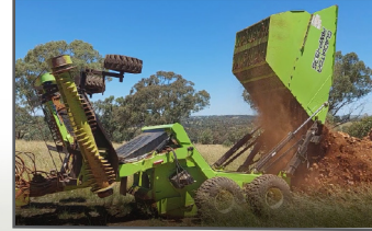
Dumping height 8' 7" (2616mm) allows for larger piles when dumping
