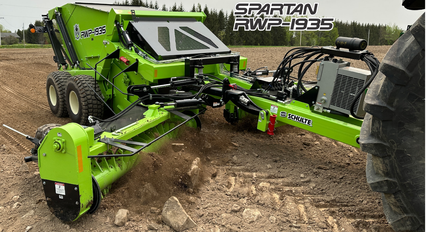
Heavy duty batt springs, 450 BNH steel reel and grate with replaceable teeth
