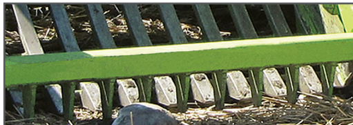
Wide grate for minimum till picking
