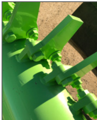
Bolt-On Replaceable Teeth
