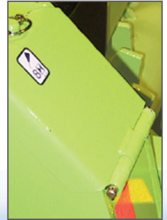
Fully enclosed final drive chain
