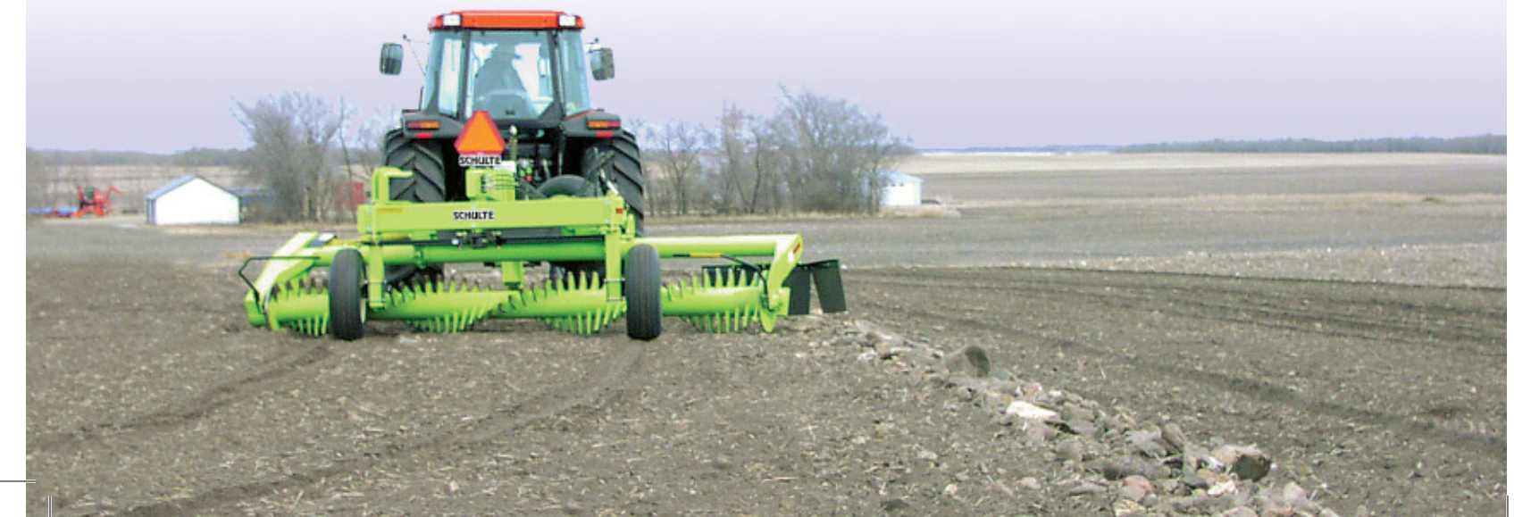
SRW-1400-H Features a hydraulic chain drive system
