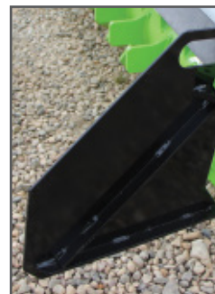
Adjustable, reversible side plates
