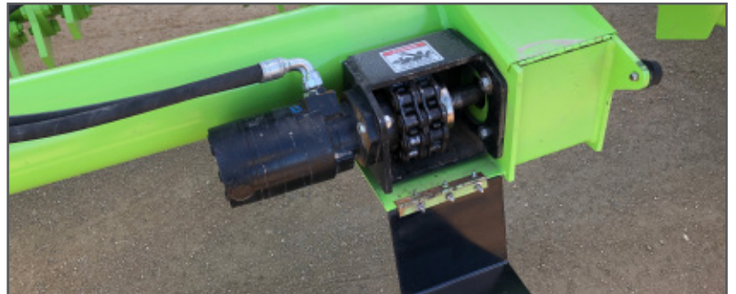
SRW-1400-H Features a hydraulic chain drive system
