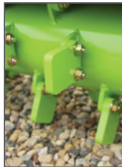
Replaceable teeth 4" & 2 1/2" 450 BHN steel
