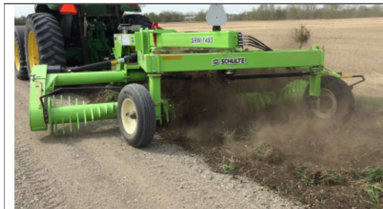
SRW-1400 doing gravel reclamation
