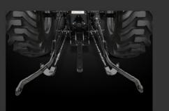
Our 3-point CAT 1 hitch has lift arm telescoping stabilizers for fast and easy implement hookup.
