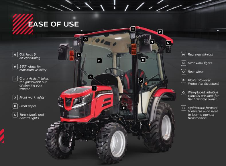
The Mahindra 2100 Series ROPS cab (Rollover Protection Structure) is designed, fabricated, and fitted at our assembly plant. It offers a comfortable ride all year round with built-in heat and air conditioning. Additionally, the glass-enclosed cab provides a 360-degree view and includes work lights, mirrors, and
