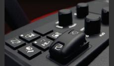
On cab models, the electronic rear hitch controls improve chore efficiency and overall productivity. Easily adjust lift speed, draft, depth, auto-raise on turns, & more.
