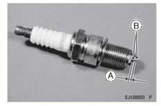
A. Spark Plug Gap B. Electrodes
