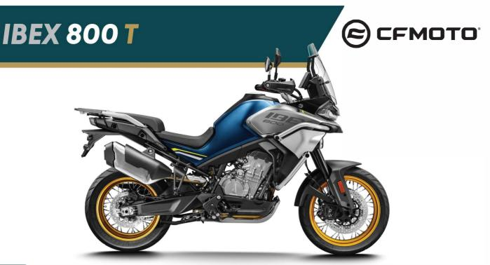
**Engine** 2-cylinder inline, liquid-cooled, 8 valves, DOHC
