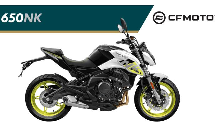
**Engine** 2-cylinder inline, 4-stroke, liquid-cooled, DOHC
