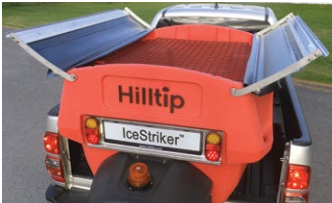
Two-piece tarp mechanism and top screen
