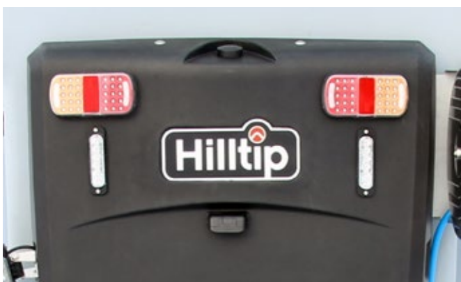
LED rear lights and strobe lights (optional)
