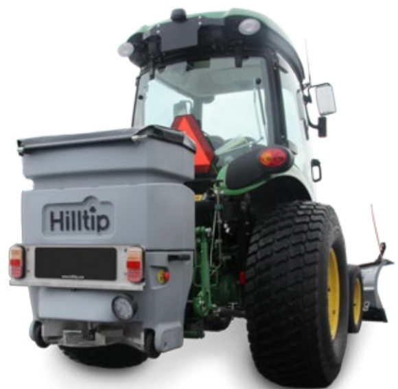
IceStriker™ 200 tailgate spreader
