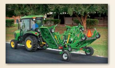
The FM20 and FM21 Series Flex-Wing Grooming Mowers feature heavy-duty frames and high flotation tires for transport. A single-action hydraulic folding wing system makes transport simple, while a SMV sign, transport safety chain, and lights are standard.
