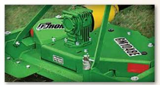
A rugged gearbox with cooling fins provides durability and reliability.
