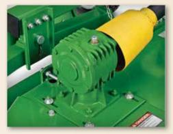
The FM21 Series Grooming Mowers feature rugged mower deck gearboxes with spiral gears that significantly reduce noise, increase endurance, and transmit more power to the cutting blades.
