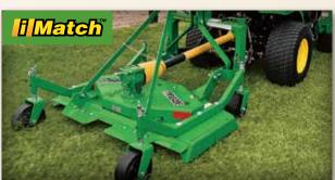
Frontier economy-duty grooming mowers can be fitted with the John Deere iMatch quick-hitch system. iMatch converts your tractor's 3-point hitch to fixed hooks and attaching points for a super-quick connection. (iMatch² hitch and implement A-frame kit sold separately.³)
