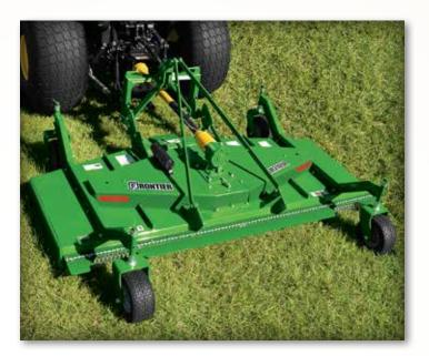
The medium-duty GM21 Series is the wider and heavier version of our rear-discharge, three-spindle mowers. Rear mounted, it's adjustable to cutting heights of 1.3 to 5.3 inches (3.3-13.5 cm). A front anti-scalping roller helps prevent scalping, while six freeswinging kickback blades make the medium-duty GM21 Series ideal for commercial use.
