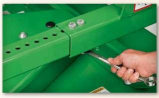
Adjust the telescoping wings to obtain the cutting width and mowing overlap you need. Simply remove the retaining bolts and roll the wings to the desired position.
