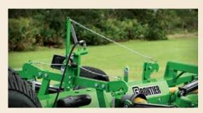
The hydraulic unlock system field conversion kit<sup>3</sup> allows the operator to unlock the wings from the tractor seat with the convenience of their hydraulic lever. It replaces the standard rope disengagement that comes with the flex-wing mower. The hydraulic unlock system is ideal for operators who fold and unfold the unit frequently to go from job to job.
