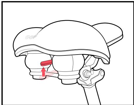
I. Pull up the lever located under the seat cushion.
