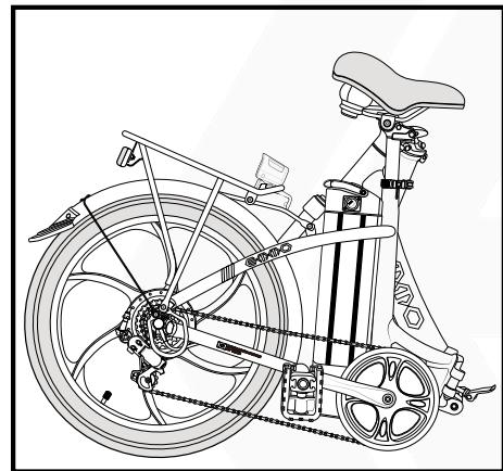
**VII.** Lift the folding lock quick release upward to unlock it.
