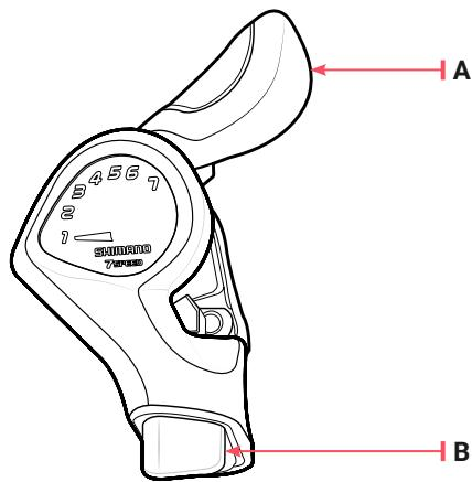
**A** Pushing the upper lever to raise the gear (smaller numbers).
