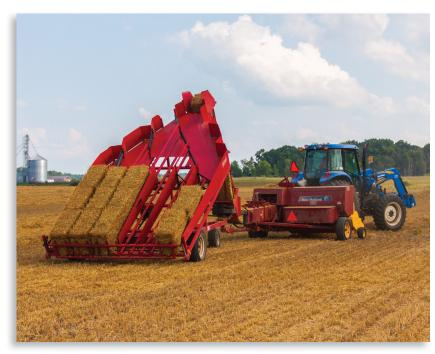
easily handle 35 to 80 lb bales, 32 to 48 inches long, allowing production of the size bale that best fits your operation. Owners of the Kuhns system have operations ranging from 1,000 to 130,000 bales per year.
