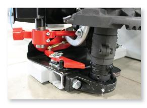
While traveling with the loaded Tie-Grabber, the operator will activate the secondary hydraulic circuit. The twine arm then rotates to the left side for the twine to be tied securely with the Rasspe™ knotter. When that is finished, the hay is ready to be deposited. When traveling to the next group the operator can return the twine arm to the right hand side.
