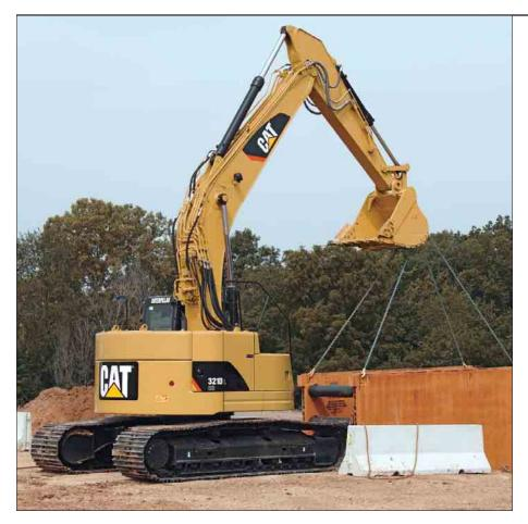
**Component Layout.** To optimize efficiency of hydraulic performance, the hydraulic components are located close together, which reduces friction loss and pressure drops in the lines.
