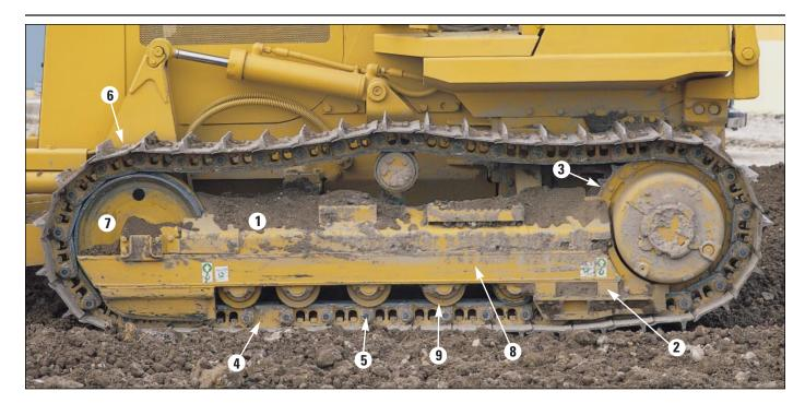
Undercarriages are designed and built by Caterpillar for long wear life and low owning and operating costs. Three different undercarriage configurations are available, allowing you to spec the tractor to best meet your job needs:
