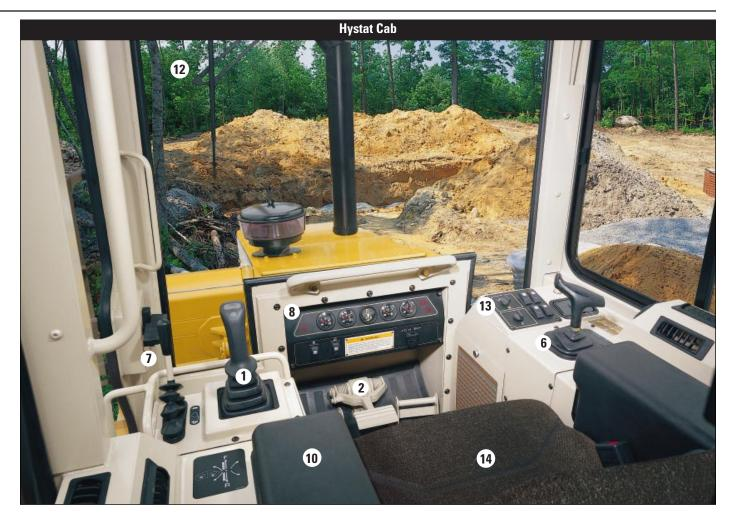
The pressurized cab is sealed to keep dust out and sound to a minimum, resulting in a quiet working environment. Nine adjustable vents keep air circulating and improve the cab's heating, optional air conditioning, and defrost/defog capabilities.
