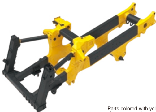
Parts colored with yellow show cast-steel components.
