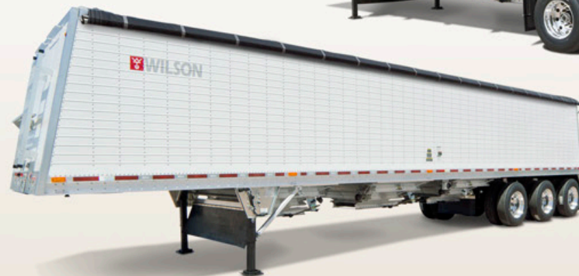
◀ DWH-550C Commander 46' long, 102" wide, 84" sides. Tri-axle and tri-hopper with third hopper discharge ahead of the rear suspension.
