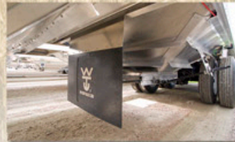
48" wide one-piece mud flap in front of rear trap. Mounted to stiffener
