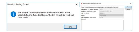
14. If the ECU **READ** matches the ECU file number, click on "**WRITE ECU**" button, read the warnings, check the items listed on screen and then click "**OK**". The flashing procedure will begin and will take approximately 5-6 minutes to flash the ECU with the new Performance Repower.
