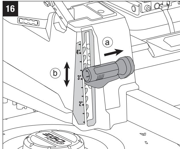
**NOTICE:** Prior to mowing, the deck should be adjusted to sufficient height to avoid stumps, rocks or other obstacles that can damage the mower deck.
