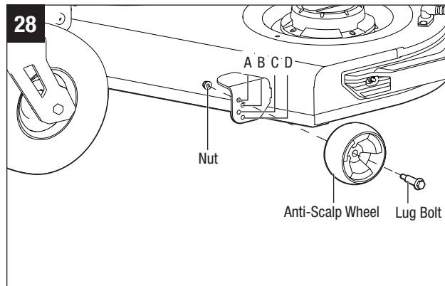
**NOTE:** One 13/16 in (21mm) wrench and one 23/32 in (18mm) wrench are required to level the cutting deck. The wrenches are not included. One mower deck leveling gauge is required and should be purchased separately.
