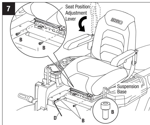
4. Use the Allen key **D** to thoroughly tighten the steel rails onto the suspension base with the remaining two socket head screws **B** (Fig. 8).
