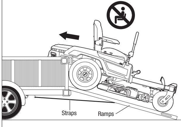
For your safety, make sure that the incline of the ramps is less than 15° whenever possible.
