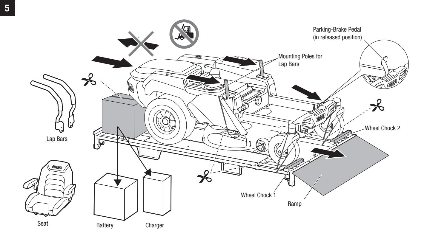
**⚠ CAUTION: Heavy object. Team push required.** At least two persons are required to push this mower off of the steel frame.
