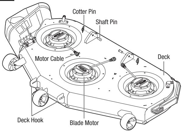
**NOTICE:** Reconnect the motor cables, ensuring that the left motor cable is connected to the left motor, the middle motor cable to the middle motor, and the right motor cable to the right motor. Left, middle, and right are marked on the cables.
