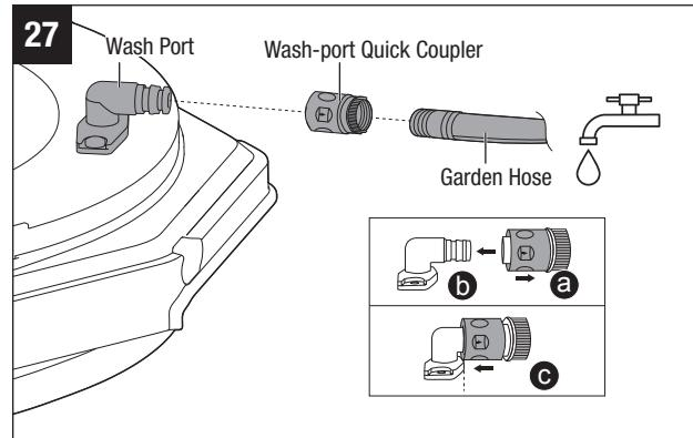
**NOTE:** When cleaning the deck using the wash port, the mower can be either in mulching or side discharging mode.
